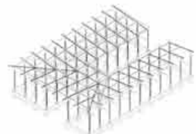
7. install ceiling rafters
