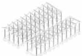
8. install wind bracing, both horizontal and vertical
